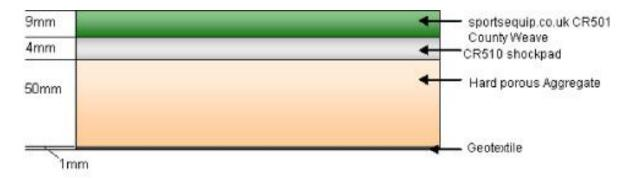
The County Weave system is a traditional non-turf pitch using a 50mm compacted hard porous base. This is laid onto an optional geo-textile layer and when levelled and compacted provides play similar to a good natural turf pitch. **sportsequip.co.uk** fit as standard a stiff load bearing base pad over the whole base to produce an even bounce and reduce base maintenance.
