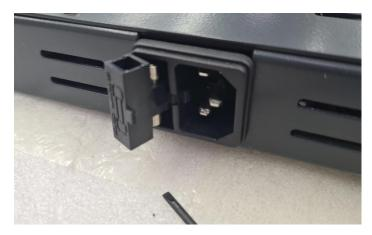
Lift fuse cover from socket and remove
