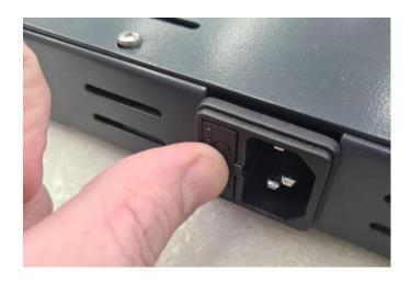
Place fuse and holder back into socket and push holder until it is level with the rear of the socket to ensure correct fitment
